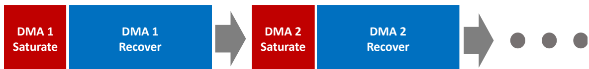
Figure 3: Progressive transitioning of district metered areas (DMAs) ensures the availability of water and human resources during the transition stage.
